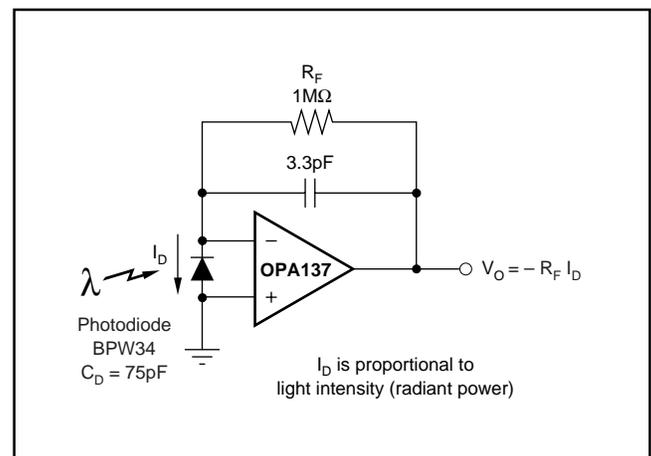
FIGURE 3. Photodetector Amplifier.
