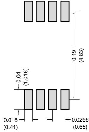
Refer to end of data sheet or Appendix C of Burr-Brown Data Book for tolerances and detailed package drawing. For further information on solder pads for surface-mount devices consult Application Bulletin AB-132.
